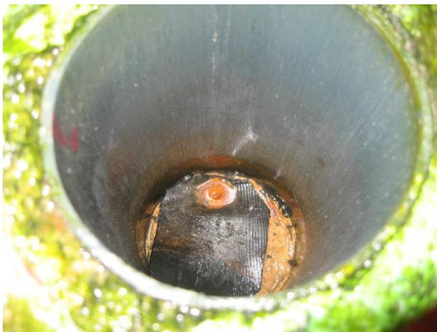
**Washer showing screw attachment, bottom of piston**
